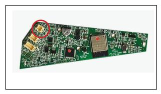
13. Connect the remaining wires to the 6-pin and 8-pin connectors on the new circuit board.
