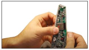
12. Connect the DFI wires to the 4-pin connector on the new circuit board.
