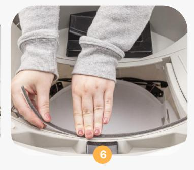
Replace the forward seal strip first, which is 13.5"L. Peel off the adhesive backing on the strip and place it along the inside of the strip guideline. Run your finger along the strip a few times to ensure adhesion.
