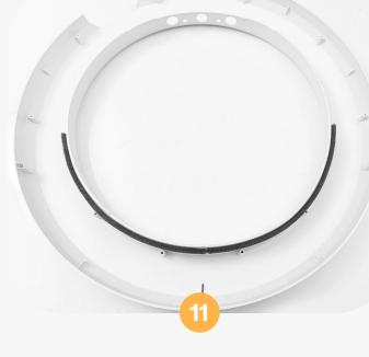
Peel off the adhesive backing on the first seal strip. Place the strip to the left of the bottom center of the bezel. Repeat with the second seal strip and place to the right.
