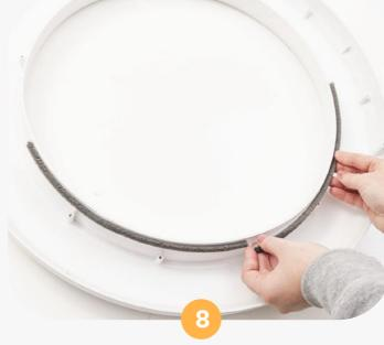
Locate the two (2) old bezel seal strips. Use a putty knife, flathead screwdriver, or your fingernail to lift the corner of the strips and peel them off.
