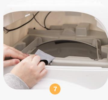
To ensure that the new seal strips adhere to the base, remove any litter and old strip residue. This can be done with some 3/8 inch strips of Gorilla Tape or another type of sturdy duct tape. Apply tape to residue, rub to adhere firmly, and pull off. Repeat around the port. Clean any residue left behind with rubbing alcohol.
