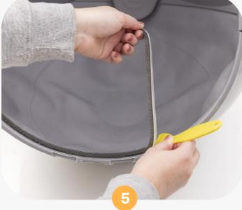
lf seal strips have already been installed here, you'll need to remove the old strip and any residue to install the new seal strip. To do this, use a putty knife, flathead screwdriver, or your fingernail to lift the corner of the strips and peel them off. You can also use 3/8 inch strips of Gorilla Tape or another type of sturdy duct tape. Apply tape to residue, rub to adhere firmly, and pull off. Repeat around the port. Clean any residue left behind with rubbing alcohol.
