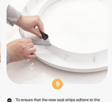
base, remove any litter and old strip residue. This can be done with some 3/8 inch strips of Gorilla Tape or another type of sturdy duct tape. Apply tape to residue, rub to adhere firmly, and pull off. Repeat around the port. Clean any residue left behind with rubbing alcohol.
