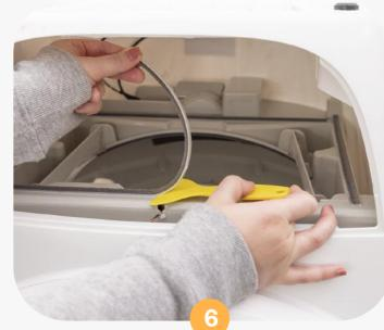
Locate the old lower waste port seal strips. Use a putty knife, flathead screwdriver, or your fingernail to lift the corner of a strip and peel off all four (4) strips.
