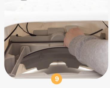
Proceed to the forward and rear seal strips, which are 13.5"L. Place the rear seal strip in front of the strip guideline, and the forward seal strip behind the seal strip guideline.
