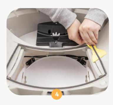
✓ Locate the old upper waste port seal strips in the base. Use a putty knife, flathead screwdriver, or your fingernail to lift the corner of a strip and peel off all four (4) strips.
