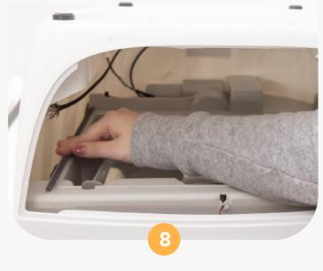
Replace the (2) side seal strips first. These are 10.25"L. Peel off the adhesive backing on the first seal strip. Start at the back, and place the strip forward along the strip guideline. Run your finger along the strip a few times to ensure adhesion. Repeat with the other side seal strip.
