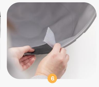
To apply a new strip, peel off the adhesive backing on the first seal strip. Adhere the first seal strip to the left side of the globe entrance. Place the strip toward the FRONT edge of the globe lip to avoid visibility when the unit is reassembled.
